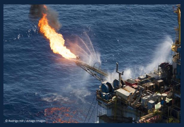
Production Testing at Echidna-1 Queiroz Galvão "Olinda Star" Semi Submersible Drilling Rig
