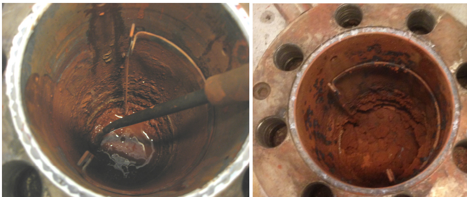
Figure 2a: Inside of the vessel to show caking at the bottom and walls after pressure leaching.
