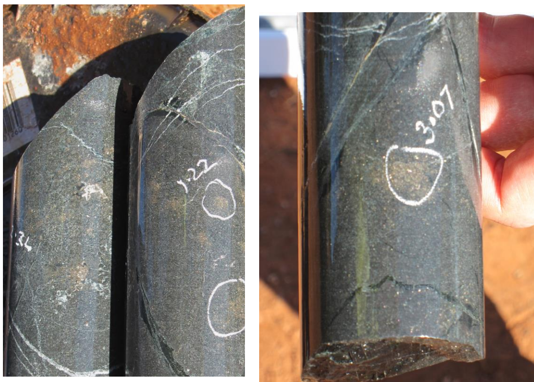
Plate 1: Disseminated and Blebby Nickel Sulphides hole RHDD0015
