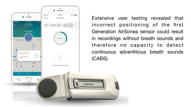
The Second Generation AirSonea wheeze detection algorithm includes a breath-screening module to ensure the device will only record and pass sounds through to wheeze analysis when breath is detected. The app warns when breath is not detected and allows the user to reposition the sensor correctly without the need to stop the recording and start again.
