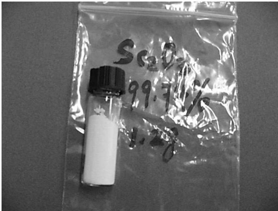
Figure 1: First high purity scandium oxide made from Syerston ores of Jervois Mining. Ltd.
