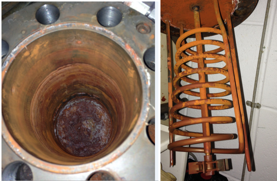
Figure 2b: The same vessel after the caking problem was solved.
