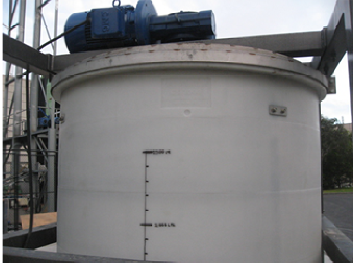
Top-stirred leach tank with a capacity to generate up to 2500L leach liquor. CSIRO has also a large filter press to carry out the solid-liquid separation.
