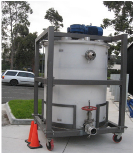
Top-stirred leach tank with a capacity to generate up to 2500L leach liquor. CSIRO has also a large filter press to carry out the solid-liquid separation.
