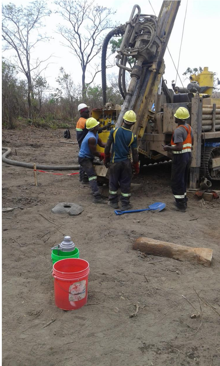
Figure 2 RC drilling rig preparing to commence drilling at the Chiwata Prospect
