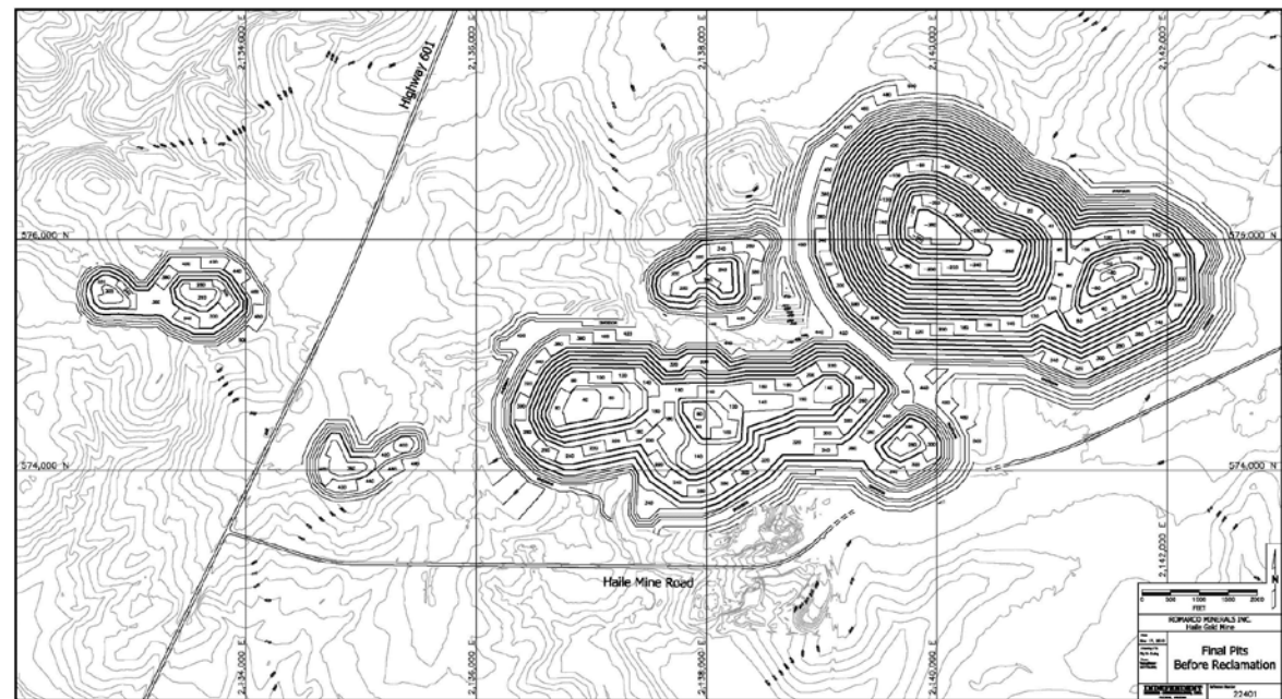
Figure 1: Final Pit Design for Orel Reserve
