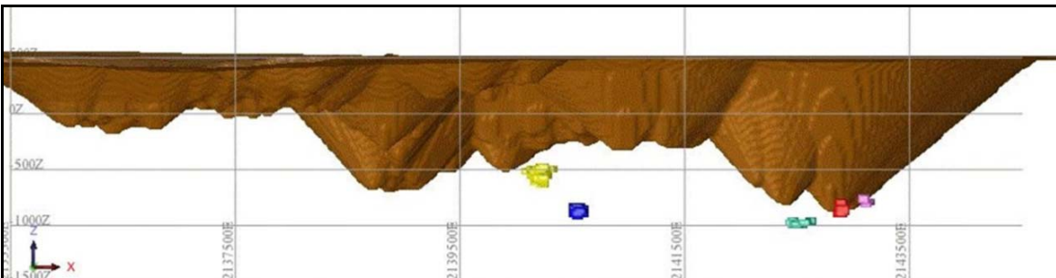
Figure 14-5: Long Section (W to E) showing location of underground stop shapes at 0.080 oz/t cut-off grade relative to $1200/oz pit shell
