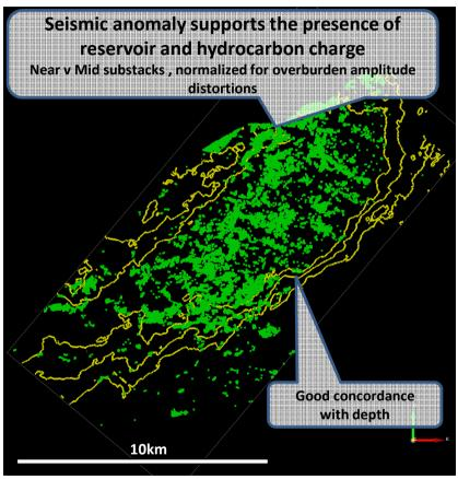
New 3D seismic and analysis provides dramatically improved resolution, and increases the confidence in the presence of reservoir, seal and hydrocarbon charge in the Elvie Prospect.
