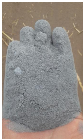
Figure 3 A sample of mineralised RC chips from the Namangale Prospect
