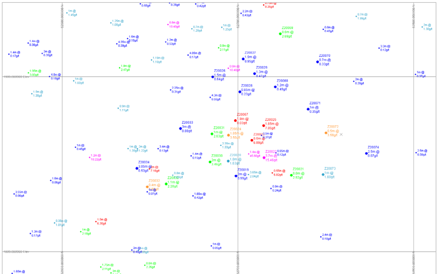
Figure 2. Long section looking west showing the location of drill holes in the Read Near and Read Extended targets. The grid is 100 m X 100 m. Holes from the current campaign have drill hole numbers. The other holes are historic.
