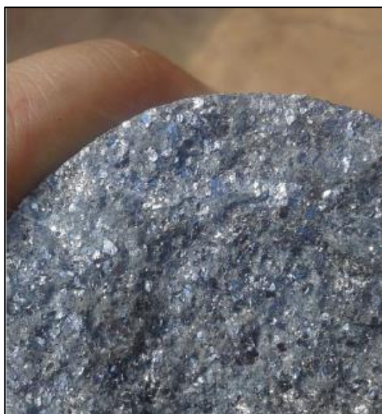
Figure 4 Diamond Drill Core - Chiwata with 3mm - 4mm graphite flakes
