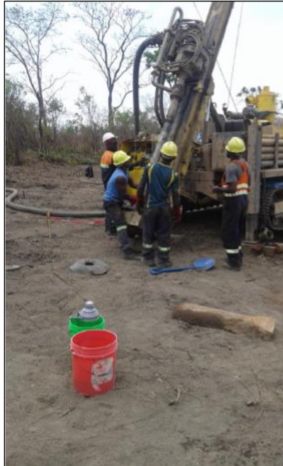
Figure 3 RC Drilling Rig Preparing to Commence Drilling at the Chiwata Prospect
