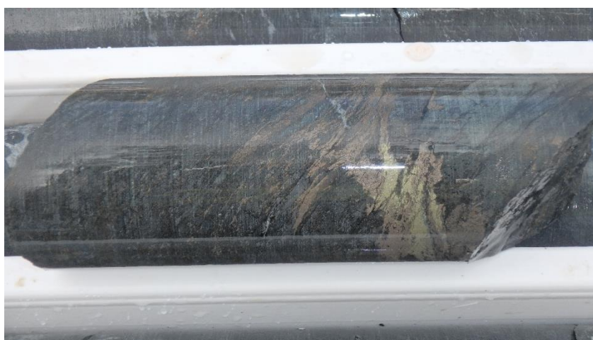
Photo 1 –Stringer of nickel bearing Massive Sulphides (~191m depth) in hole RHDD0023
