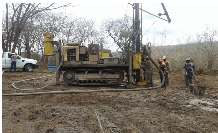
Figure 5 The RC Drilling Rig in Operation at the Namangale Prospect.
