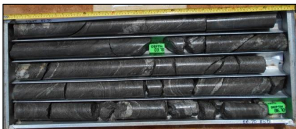
Figure 5 Diamond core from NMDD0002 from 41.15-45.75 (top left), NMDD0004 from 45-49 (top right), NMDD0001 from 82.2-86.7 (bottom Left) and NMDD0004 from 49.4 - 53.7m (bottom right)
