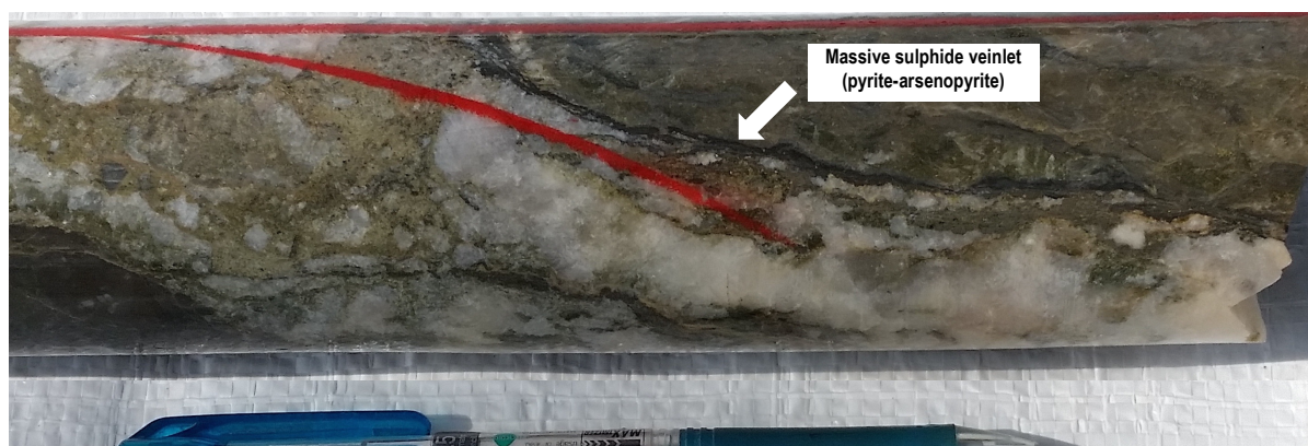
Figure 2: Sample from CHRCD002 at depth of 117 metres. Note sulphide veinlet on contact of epithermal vein / breccia unit.
