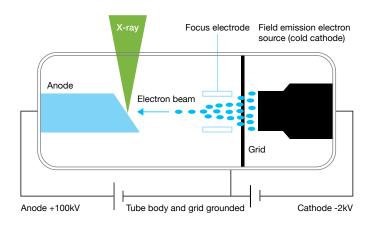
An additional benefit of a CNT electron emitter is that the electron beam is pre-formed by the process of field emission from the CNT tips to the extent that it is possible to change the path of the electron beam with a voltage on a focusing electrode through which the beam passes and thus change the size of the focal spot on the tungsten anode. The size of the focal spot can thus be adjusted to optimise image quality for each exposure.
