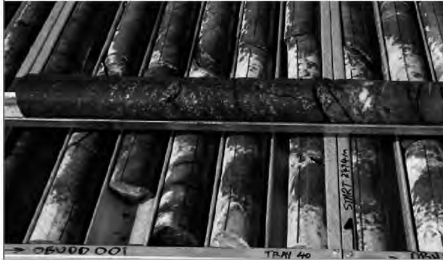
Figure 10 OBUDD001: Massive Magnetite-Chalcopyrite at Base of Feeder Structure (0.9m @ 4.5g/t Au and 2.6% Cu from 256.4m depth)
