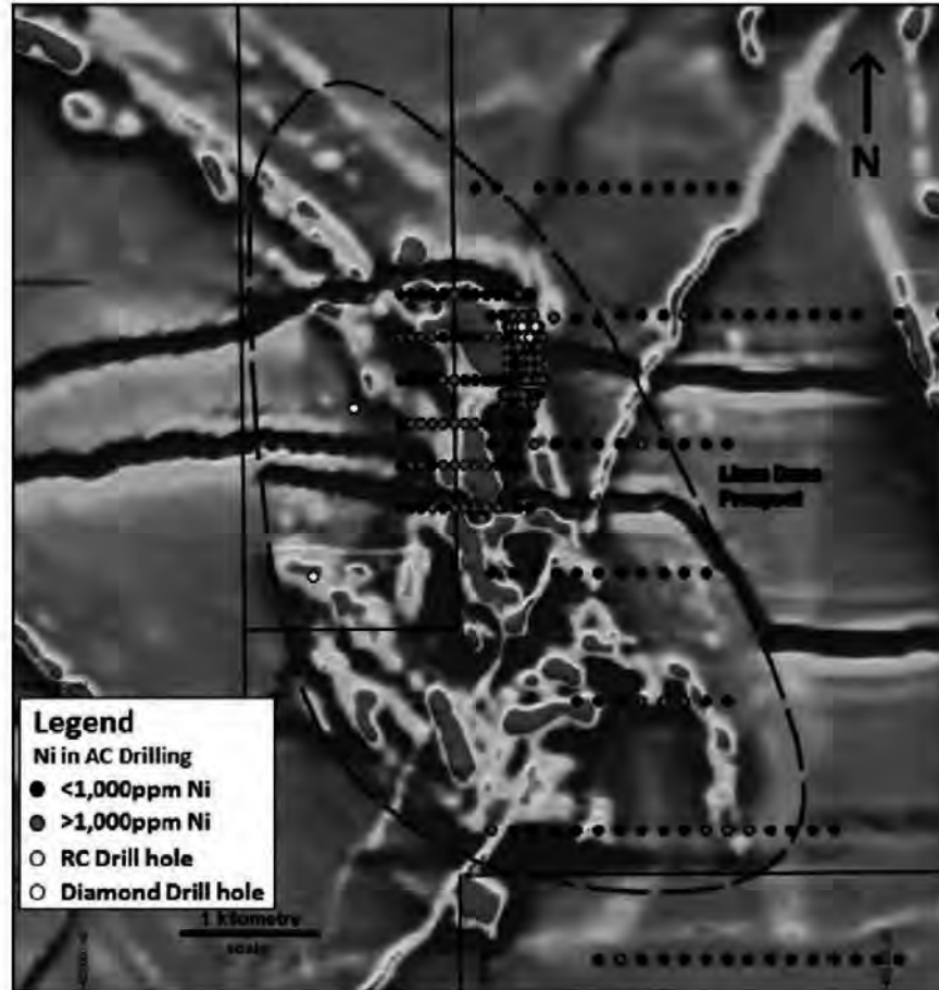
Figure 11 Lisa’s Dune Prospect: Nickel in Aircore Drilling on Aeromagnetic Image with RC and Diamond Drill Holes
