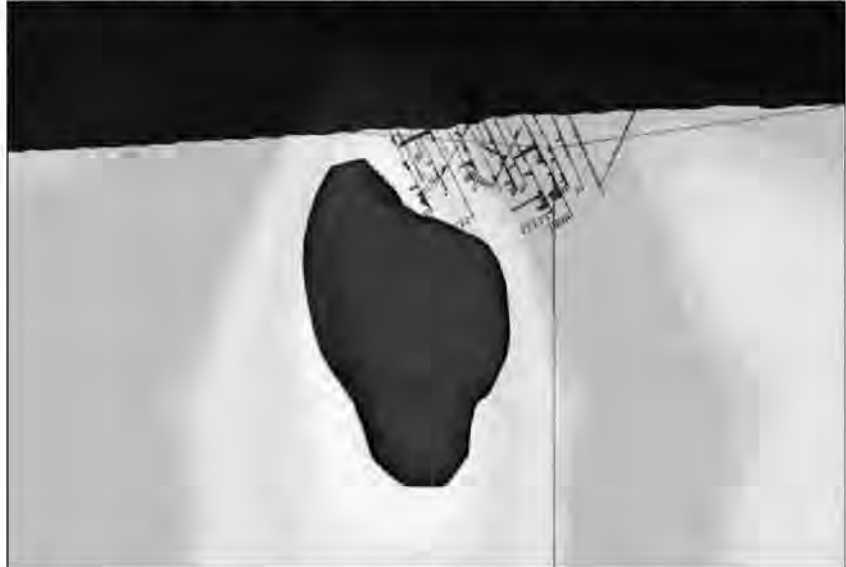
Figure 8 Burns Prospect: 3D Inversion Model of Ground Magnetic Data (red shape: 90 x 10 -3 SI Isosurface) with RC Drilling (view from below surface and to the northeast)
