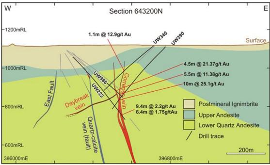
Figure 4: Geological Section, Correnso Project (643200mN)
