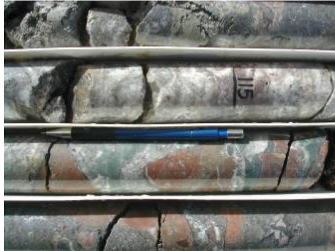
Figure 5: Zone of strong lead-zinc mineralisation in PD 64. Dark grey is galena, pale yellow is pyrite/chalcopyrite and white/grey is quartz. Original host conglomerate is reddish orange colour.
