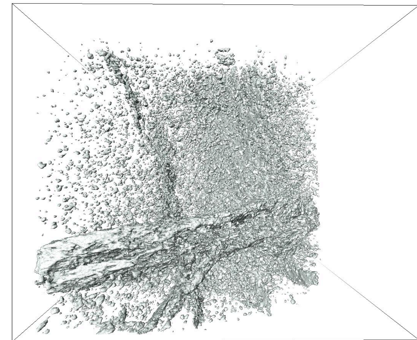
Movies of 3-d 'Tornado' scans of Nunasvaara graphite ore. Field of view = approx 5cm width.
