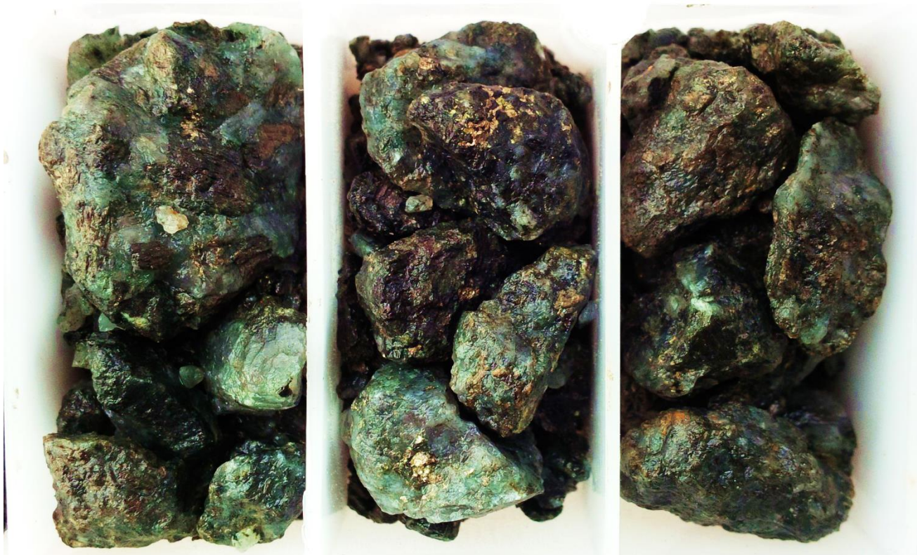
Figure 3. RC samples from SFRC0511 at Centauri, showing magmatic sulphides in mafic-ultramafic host rock.
