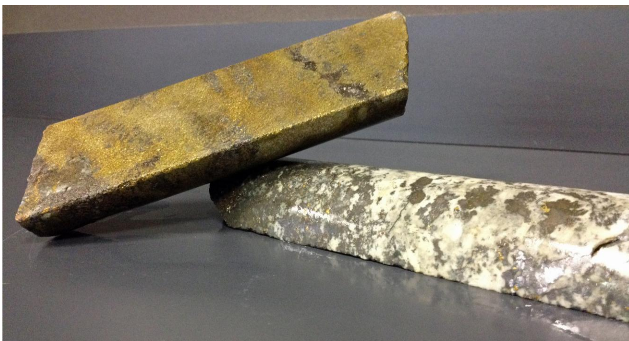
Figure 1. High grade polymetallic mineralisation from underground drilling completed in August 2013 (Top: KUPH095 75.6-75.8m and Bottom: KUPH095 88.55-88.7m).
