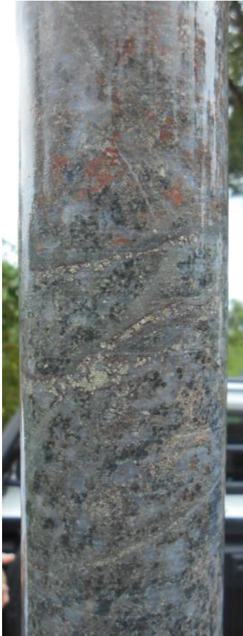
Figure 4: PRM001 - portion of 1m interval from 24.35m drill depth with sulphide mineralisation associated with strong hydrothermal alteration.
