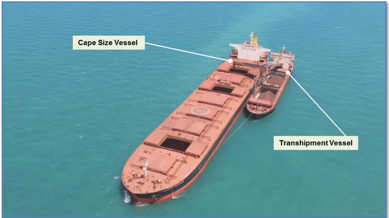
Figure 4: Transhipment Vessel in Operation
