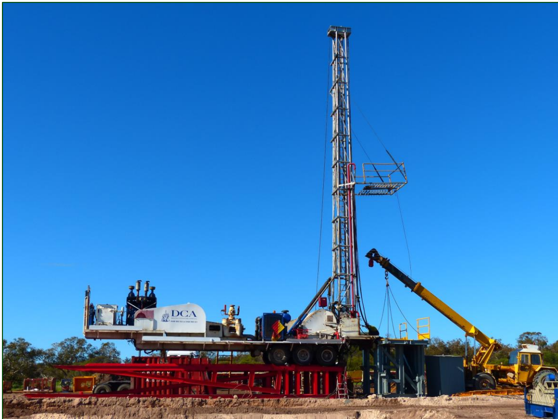
The DCA Rig 7 derrick being jacked into place over the platform
