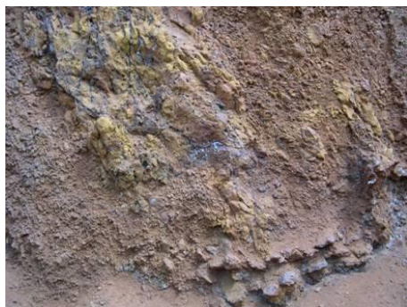
Run-of-mine siliceous ore, yellow-brown goethite and coarse silica 0.7% Ni
