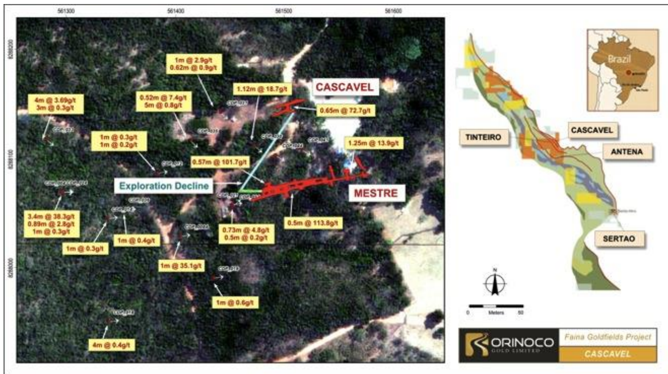
Figure 5. Location of Cascavel exploration decline. The proposed exploration decline (represented here in light blue) is a total of 90m in length. The results reported in this announcement represent the first 20m of that decline.
