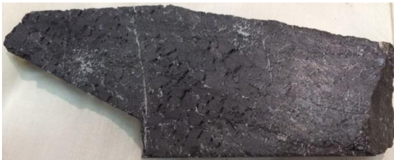
* High-grade massive V-Ti-Fe mineralisation from diamond drill hole GDH 903. Refer to full JORC Resource Table on Slide 10.
