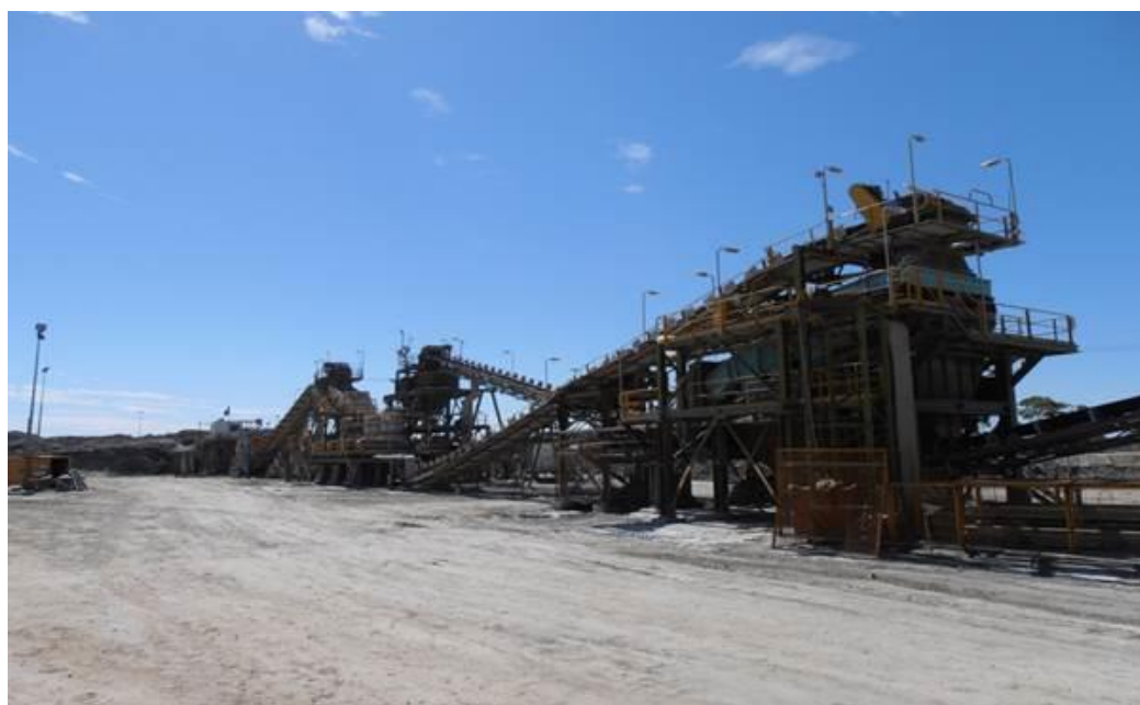
Figure 2: SIGM heap leach 3 stage crushing and screening plant (courtesy SIGM)
