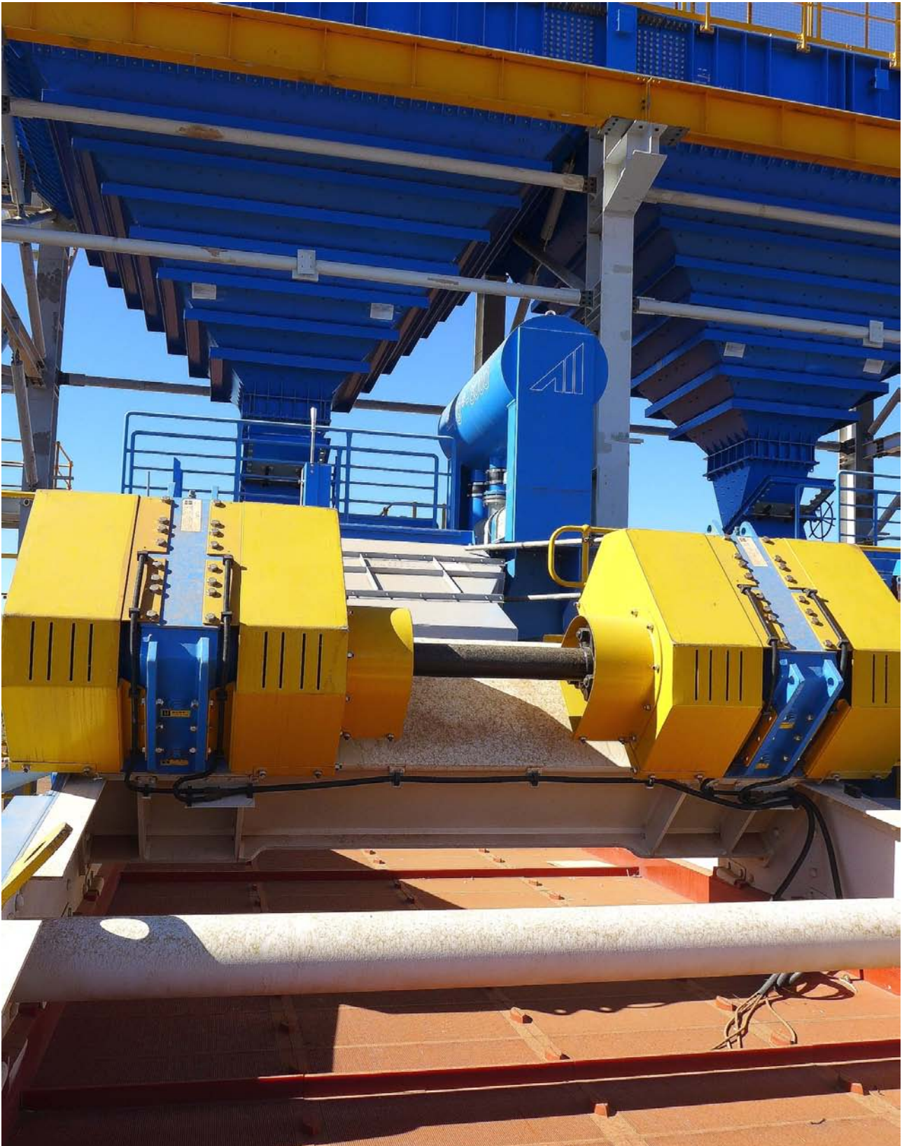
Figure 9: Gravity Jig Building - feed bins (above) and close-up of lights screen (foreground).
