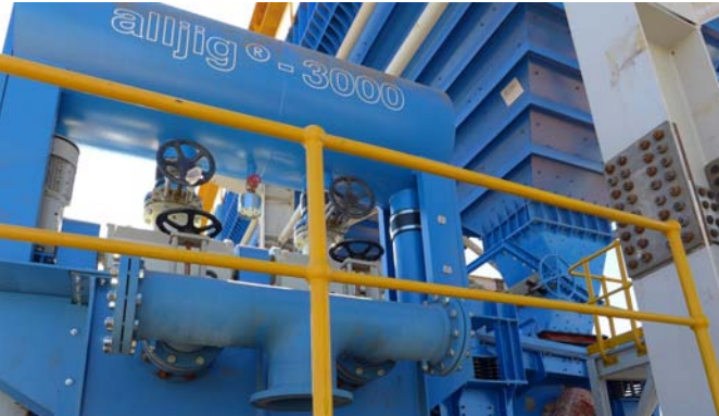
Figure 7: Gravity Jig Building - from top to bottom; native copper metal screens, feed bins and light screens and continuous alljig® units (left and right)
