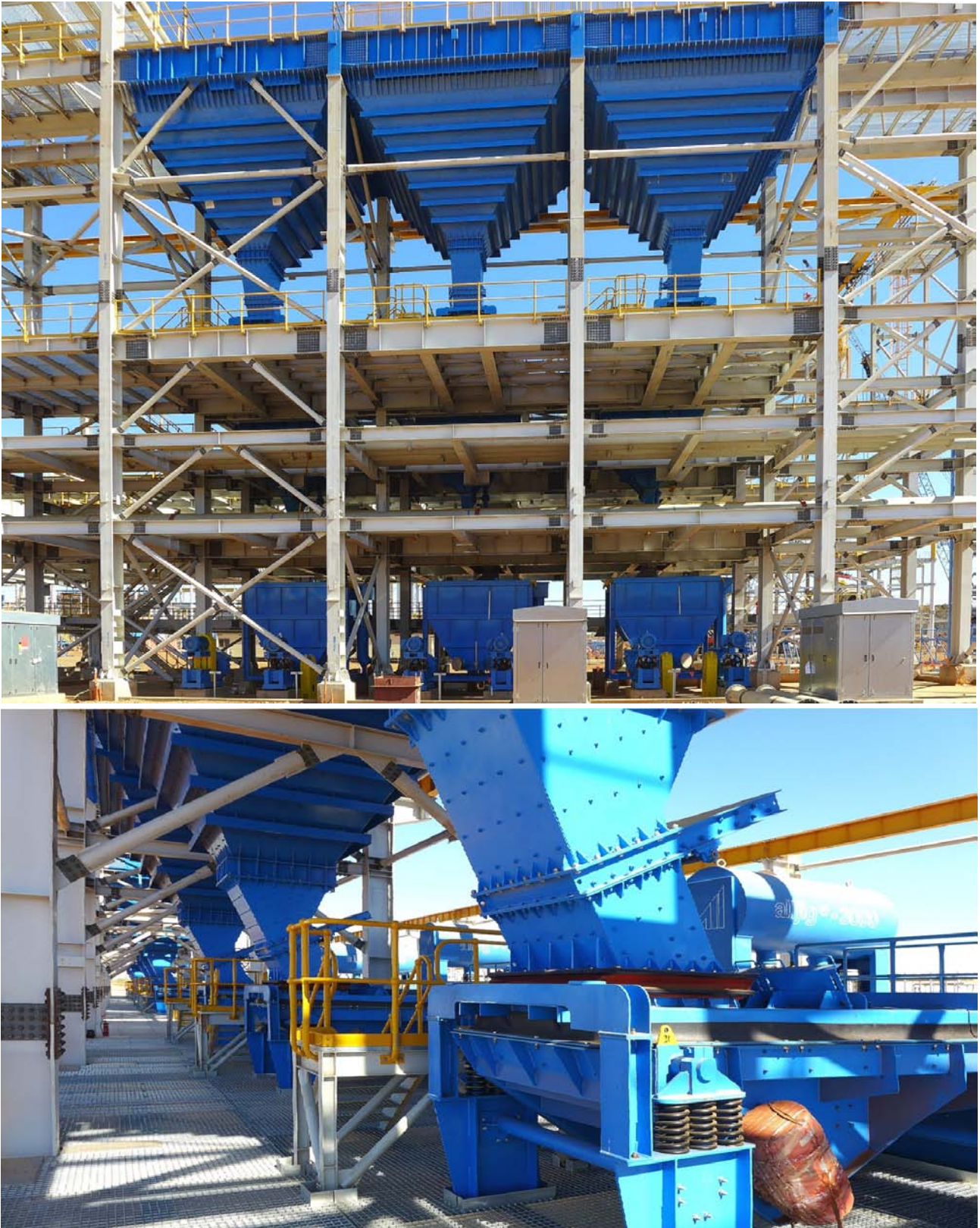
Figure 8: Gravity Jig Building - Top image; feed bins (top), screen on middle floors and pump-boxes on ground floor. Feed chutes into ore jigs.
