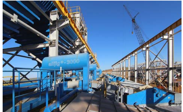
Figure 7: Gravity Jig Building - from top to bottom; native copper metal screens, feed bins and light screens and continuous alljig® units (left and right)
