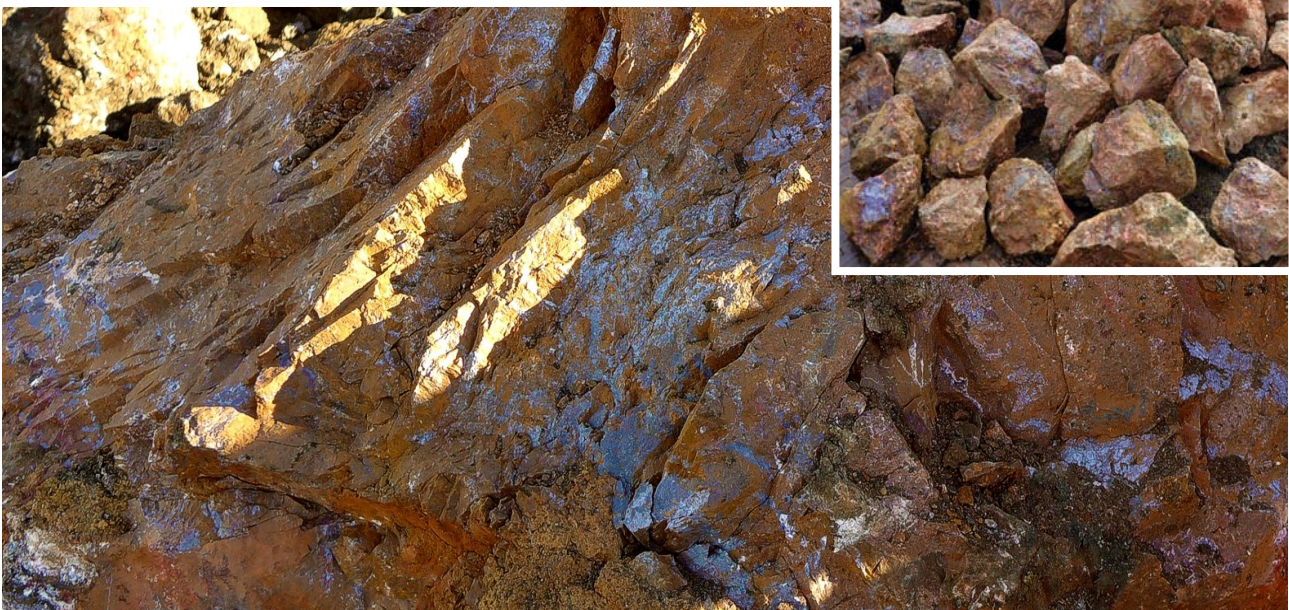
Figure 23; high-grade copper ore from the LM1 Pit - iron-rich yellow jaspilite rock matrix impregnated with massive and vein infill chalcocite (79.9% Cu), massive cuprite (88.8% Cu) and fine to coarse native copper species (99.65% Cu) - inset shows similar jaspilite after crushing through the mobile crusher, accessed in the original box-cut pit.
