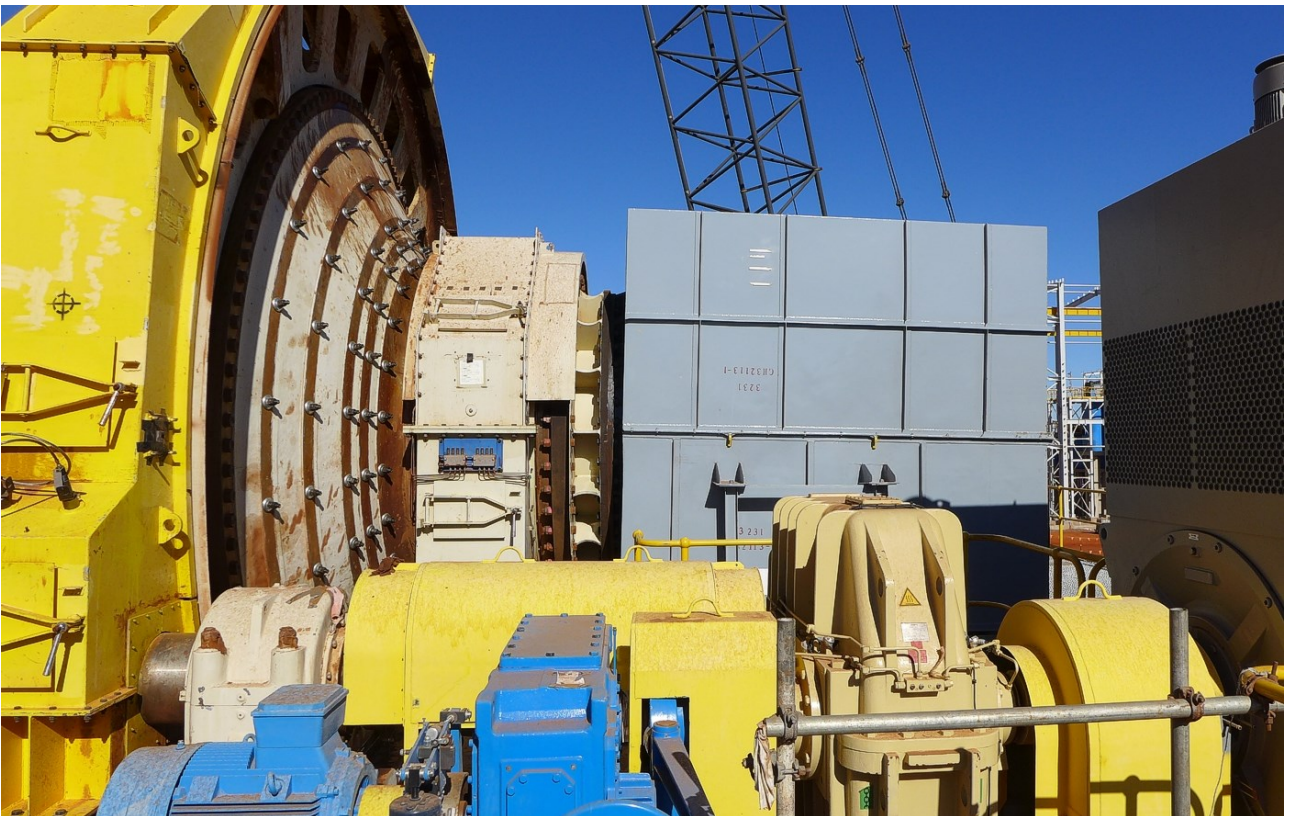
Figure 10: Ball Mill feed chute (above) and drive-train and trommel screen unit (grey box - centre)
