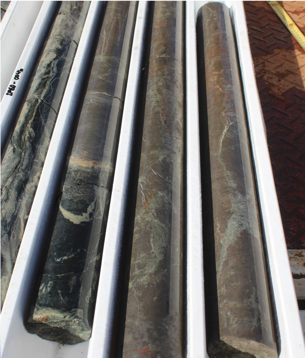
Figure 1. Massive nickel-copper sulphide intersection at Taipan with accompanying platinum and palladium.
