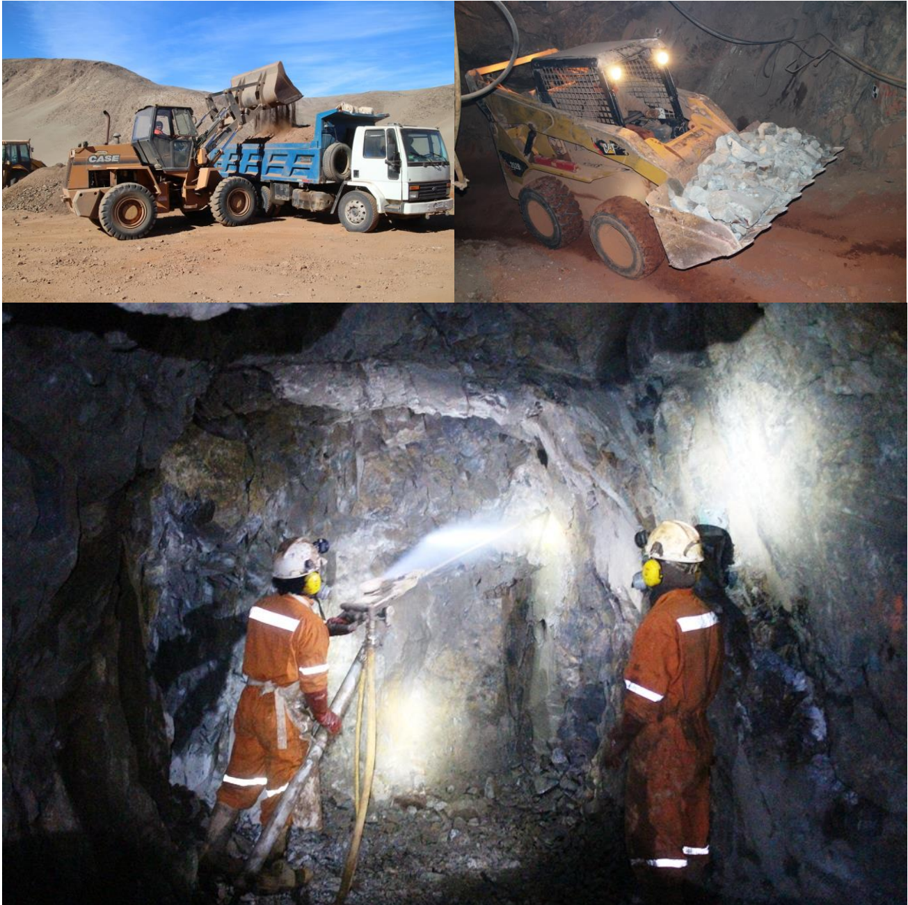
Figure 4 – Mining activities at Panga, top left – truck loading, top right – underground bobcat, bottom – airleg drilling level 956S development face.
