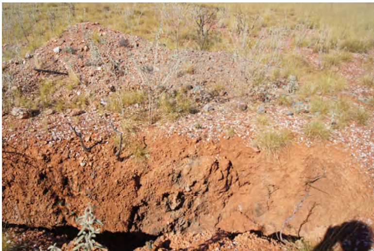
Trench with abundant secondary copper boulders from altered shear zone.
