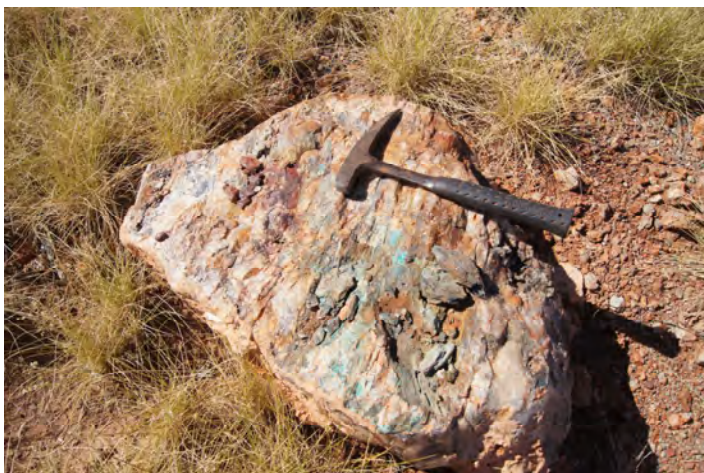
Quartz-carbonate boulder with secondary copper mineralization
