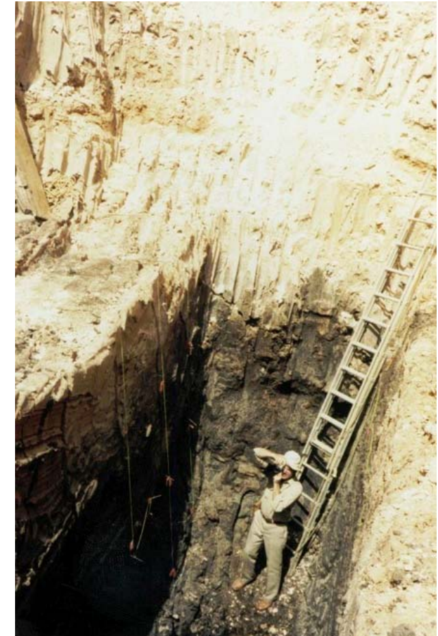
Test pit dug by PNC in the 1980s showing lignite ore and free dig nature of material
