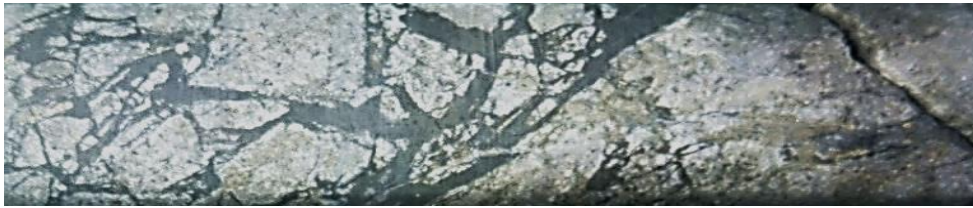
Figure 2a) CH-DDH012 at 516m: Tourmaline (high temperature alteration mineral) brecciation of locally phyllic-altered monzonite intrusion with sulphides.
