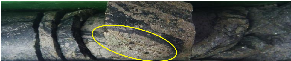
Figure 2b: CH-DDH012 at 517m: Intense brecciation of phyllic-altered monzonite with tourmaline and sulphides. As is the case in Figure 2a) the tourmaline and sulphides are closely associated. Banded fine-grained disseminated sulphides with sericite are circled.
