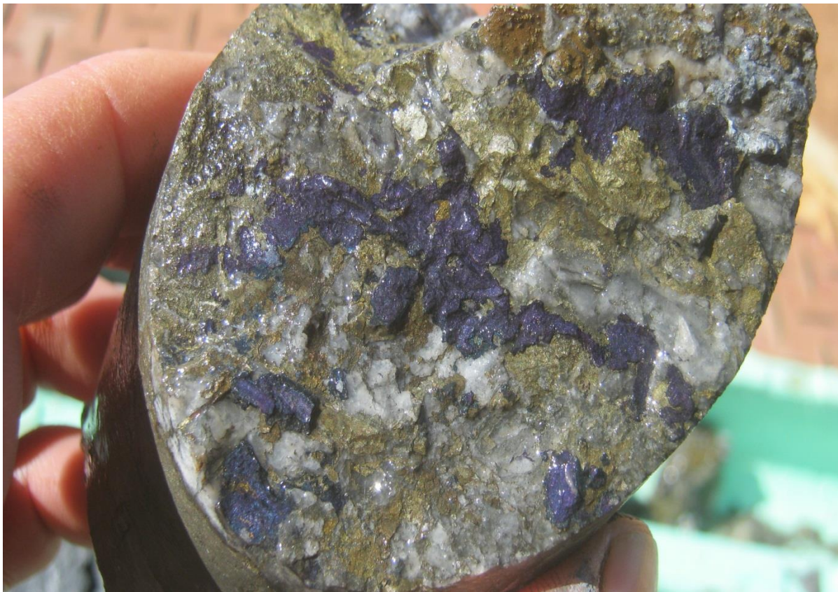
Figure 3: DD14IL175 Chalcopyrite / Bornite mineralisation at 352 metres
