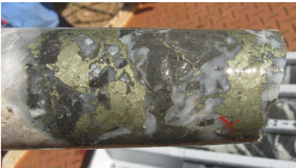
Figure 4: DD14IL14 Chalcopyrite mineralisation at 451 metres
