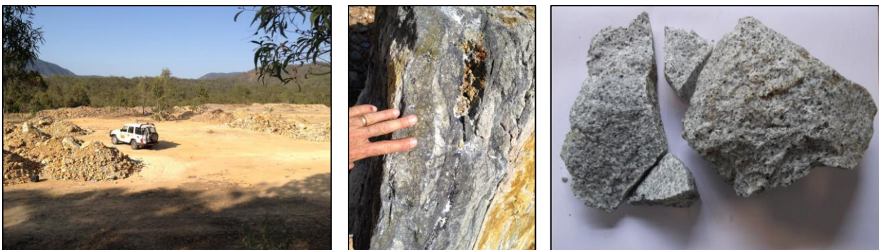
Figure 14: Frampton stockpiles, typical grade carrying shear material and typical barren wall rock.
