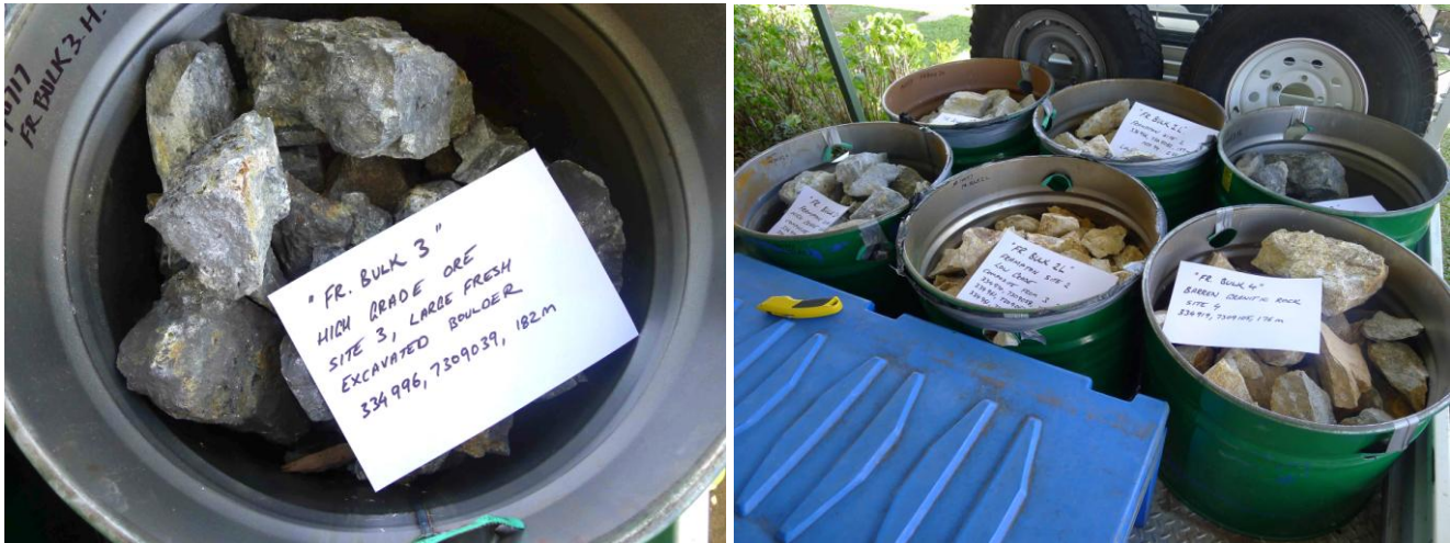
Figure 9: Portion of the final bulk sample visibly separated into various grade ranges.
