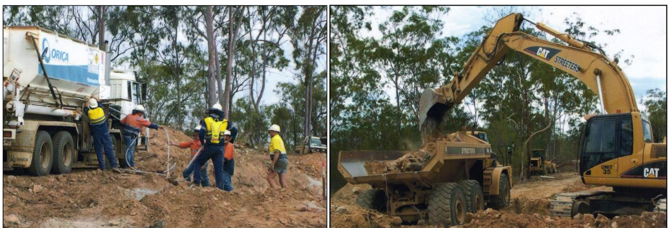
Figure 16: Prior operations charging blast holes and mining with excavator and trucks at Norton mine.
