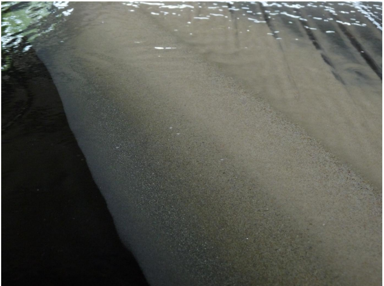
Figure 3: Clearly distinct separation of high and medium grade concentrate streams from waste.
