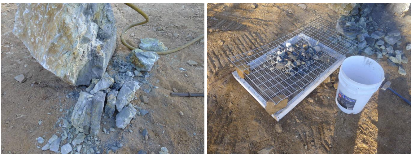
Figure 8: Size reduction and course screening of the larger, fresh, higher grade carrying boulders.
