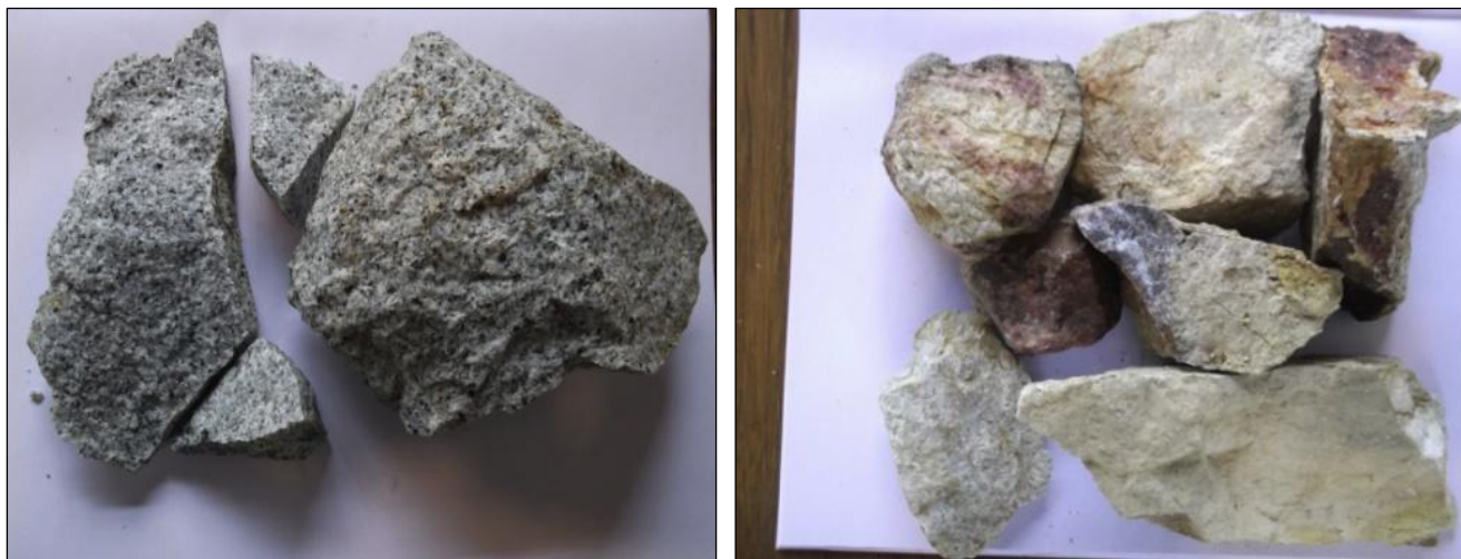
Figure 4: Typical barren granitic wall rock and low grade waste shear material.
