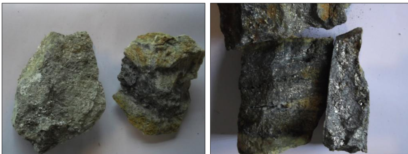
Figure 5: Typical medium grade shear material and high-grade shear material.
