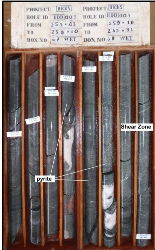
Figure 16: Hicks Drill Core: Quartz Veining Adjacent to Shear Zone (258.0m-259.0m: 1.0m grading 16.1g/t gold)
