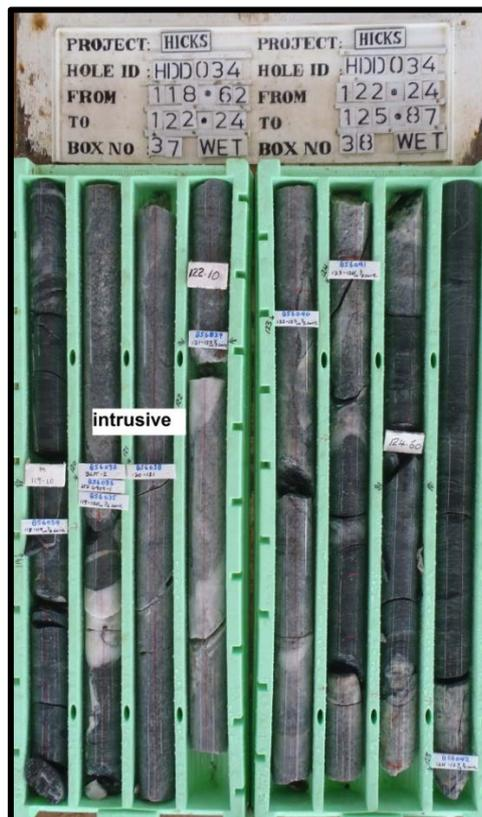
Figure 17: Hicks Drill Core: Quartz Veining Associated with Felsic Intrusive (119.0m - 125.0m: 6.0m grading 2.7g/t gold)
