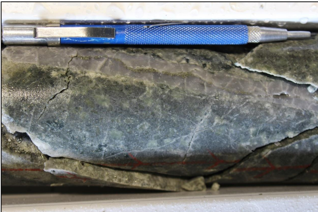
Photo 4: Typical porphyry 'B' quartz vein with sericite selvage and pyrite core in SMD001 at 390m.
