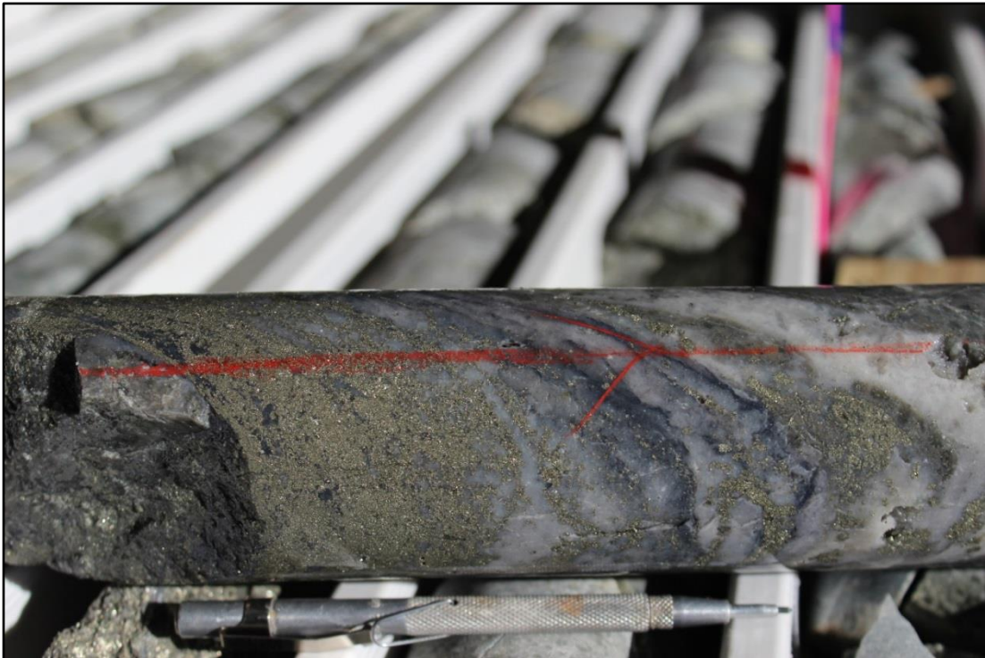
Photo 3: Typical porphyry quartz sulphide 'D' vein with pyrite, chalcopyrite, molybdenite and sphalerite in SMD001 at 381m.
