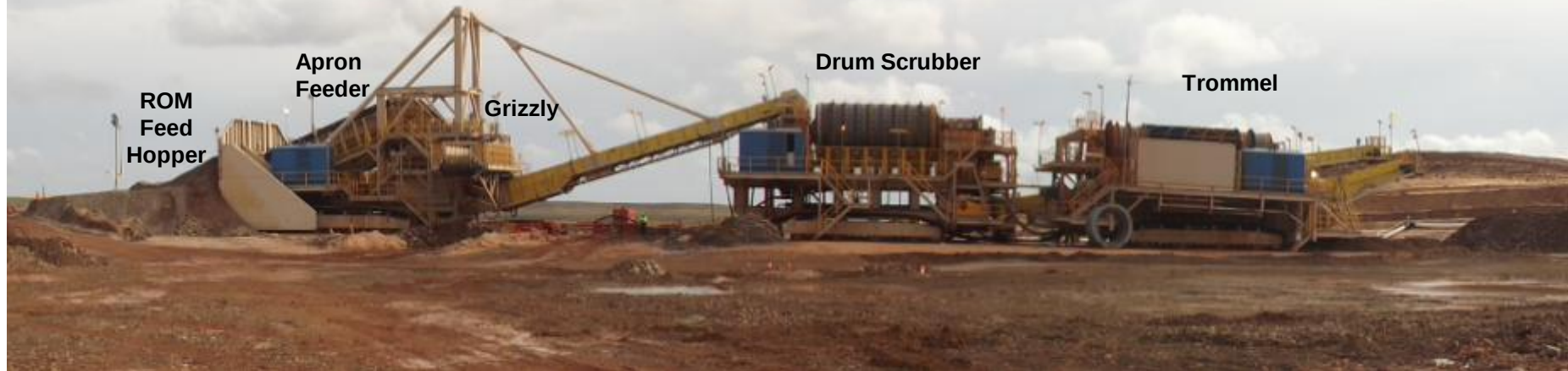
Wet Concentrator Plant
