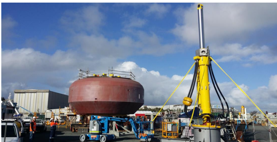
CETO Buoyant Actuator and Pump assembly at onshore test site at Henderson, Western Australia
