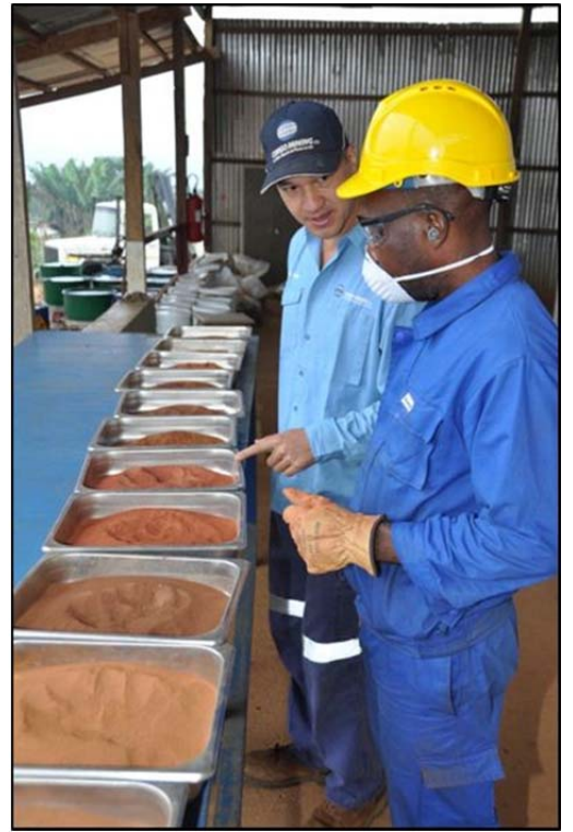
Figure 5: Preparation of trench samples at the Mayoko Sample Preparation Laboratory
