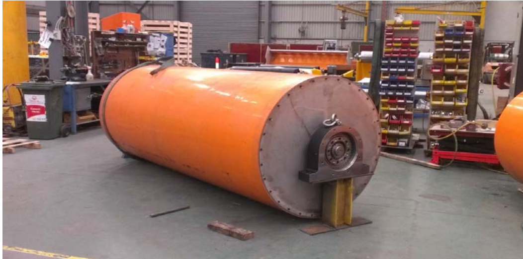
Photograph showing magnetic separator drum manufactured for Windimurra in Melbourne
