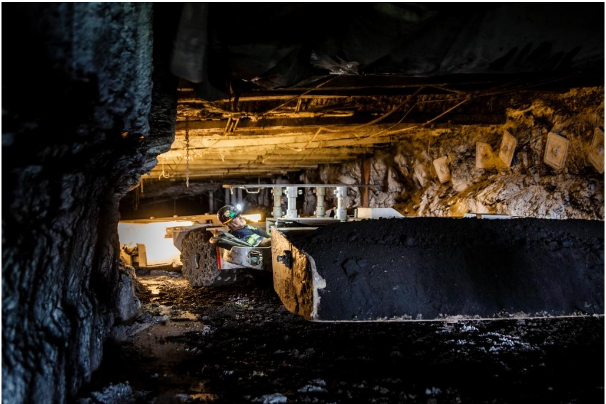
Figure 5. Attila's coal scoop transporting coal out of the Coke No.1 Mine
