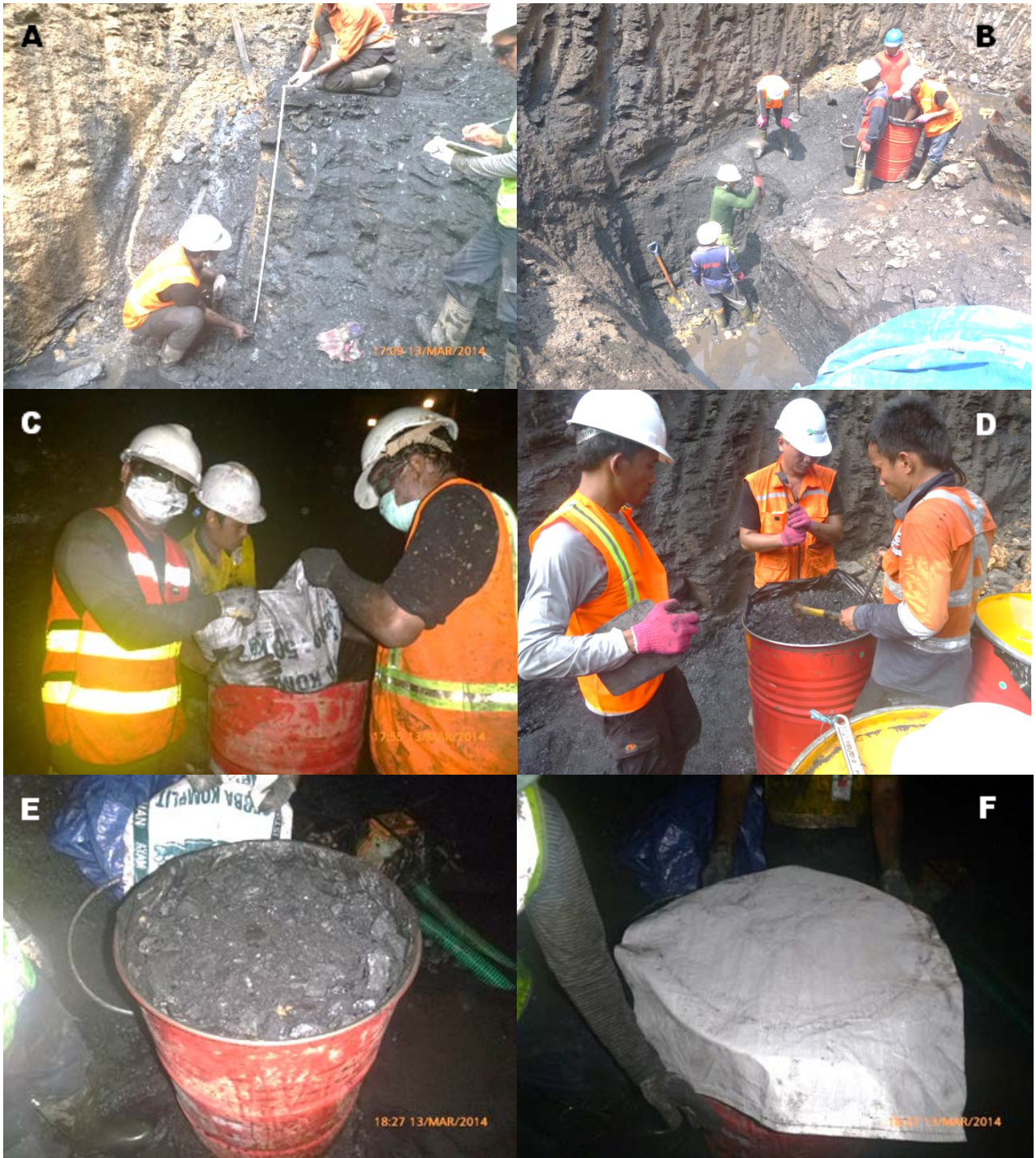
Figure 5: Coal Test Pit Sampling Process.
