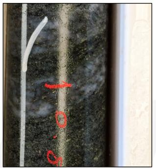
*Figure 3:* Strongly aligned pyrite chalcopyrite associated with quartz veins in a garnet bearing granulite gneiss. (14SHDD06 455.8m)
