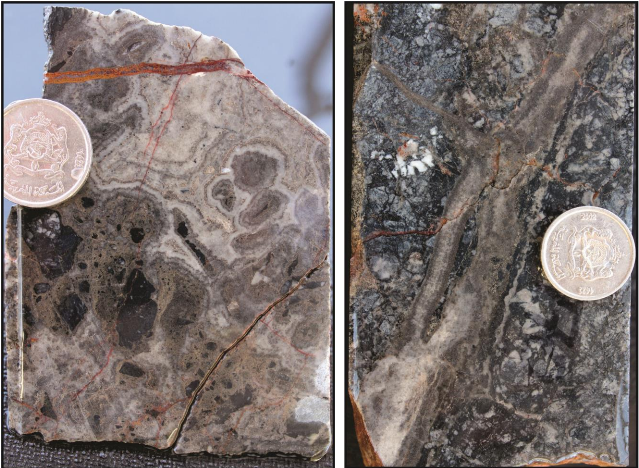
Figure 3: High grade HQ core samples from WZGTD004 returning 1m @ 10.67%Sn from 40.5m
